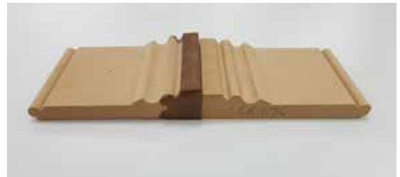
This image shows swelling to a profile when the base of the Moisture Resistant MDF moulding was exposed to water for just 24 hours!
